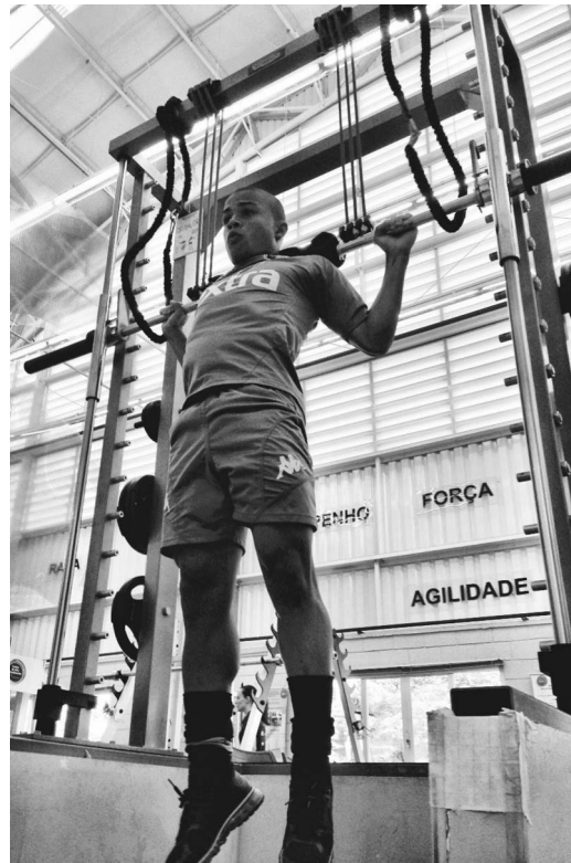
Figure 1. Illustration of the elastic band system attached to the Smith machine bar used to increase bar velocity.
